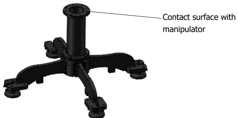
Figure 6-3 Diagram of manipulator base structure
